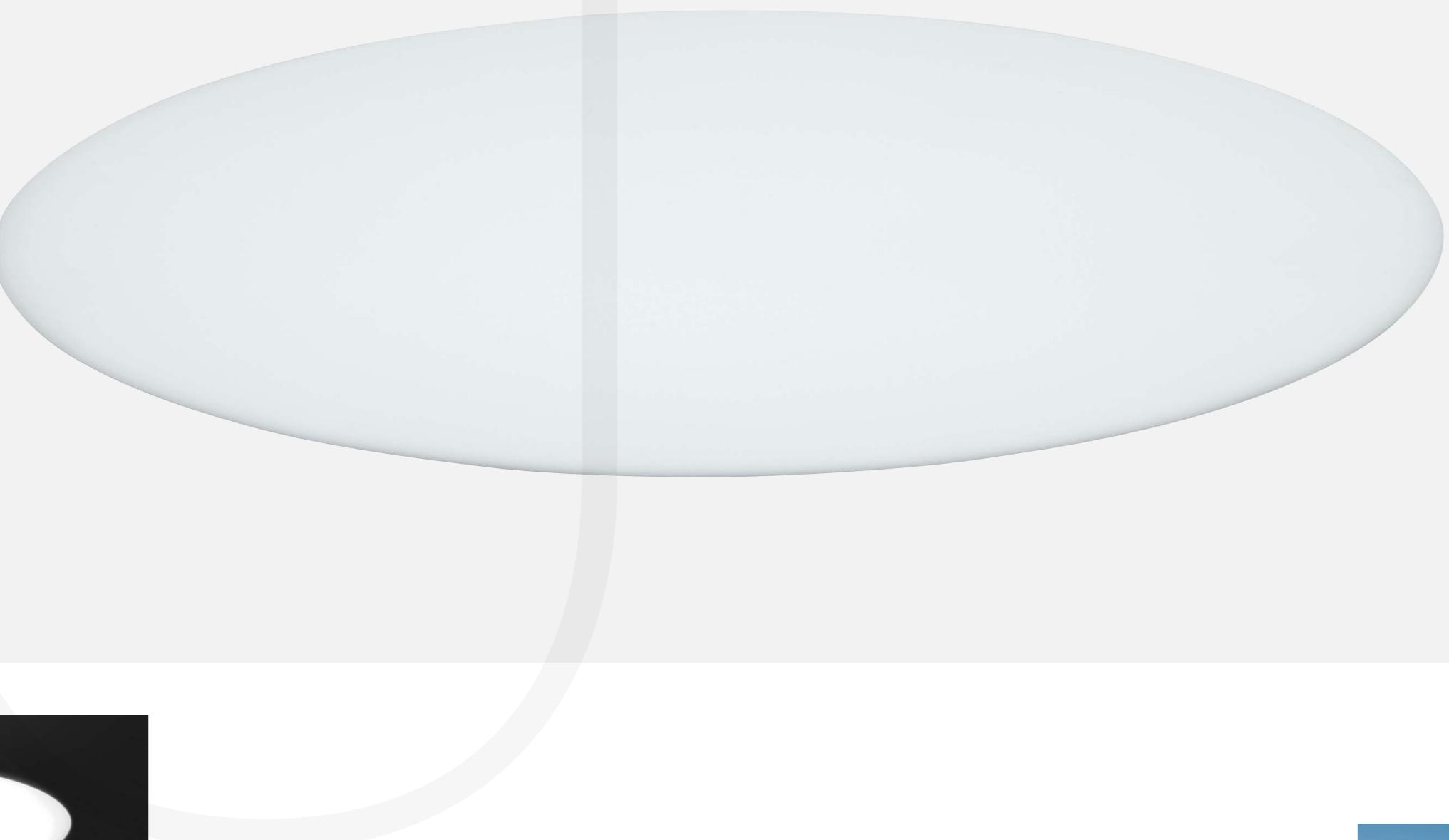
**ALASTAR C TRIMLESS** (606 mm diameter) allows you to create a look where the 110° beam angle illumination (7200 lm in CCT 4000 K, 6950 lm in CCT 3000 K) is emitted directly from the ceiling. There is no frame and the optical surface of the luminaire sits flush to the ceiling surface. ALASTAR C TRIMLESS comes with CRI 80+ Ra, a power consumption of 73 W, and the choice of a FIX or DALI dimmable driver.
