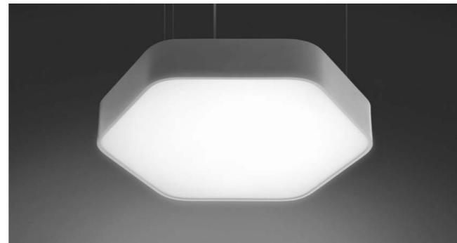
**HEX** is, as the name suggests, is a hexagonal luminaire that can be built up into an interesting honeycomb design consisting of several HEX luminaires. Available in 33 W (3200 lm at CCT 4000 K, 3150 lm at CCT 3000 K) or 65 W (6400 lm at CCT 4000 K, 6100 lm at CCT 3000 K) versions, both with CRI 80+ Ra, HEX can be equipped with a FIX or DALI dimmable driver. Each luminaire weighs 11 kg.
