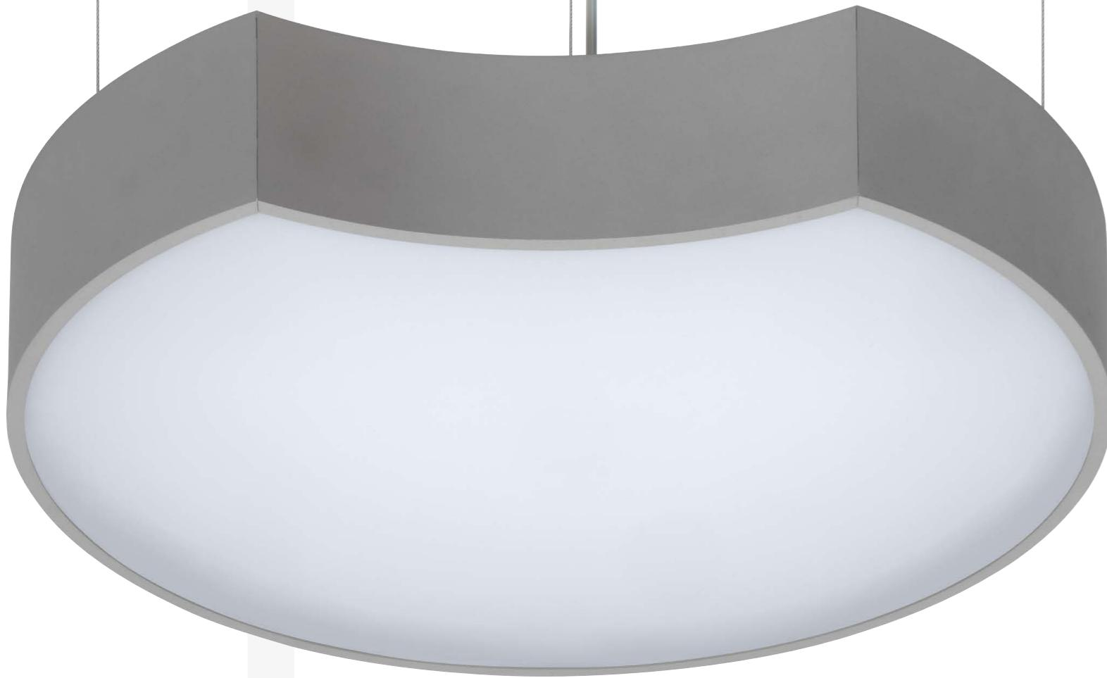
**LUNAE** looks like an almost full moon and allows for the connection of these circular forms into a vast array of designs. Available in 37 W (4100 lm at CCT 4000 K, 3900 lm at CCT 3000 K) or 74 W (8200 lm at CCT 4000 K, 7800 lm at CCT 3000 K) versions, both with CRI 80+ Ra, LUNAE can be equipped with a FIX or DALI dimmable driver. Each luminaire weighs 8.7 kg.
